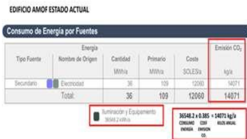
Figure 7. Result CO 2 emission. AMOF-Current State Building, Miraflores
