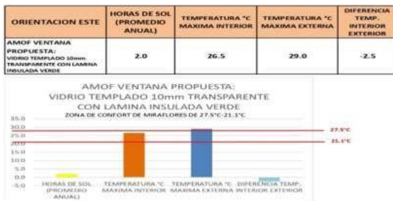
Figure 11. Thermal result. AMOF building- Proposal, Miraflores.
